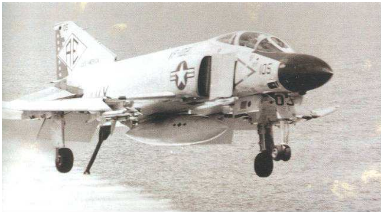
Above: Diamondback F-4J Phantom coming in for landing with an empty fuel tank and unused Sparrow and Sidewinder Missiles (Photo: RADM Peter B. Booth Collection)
